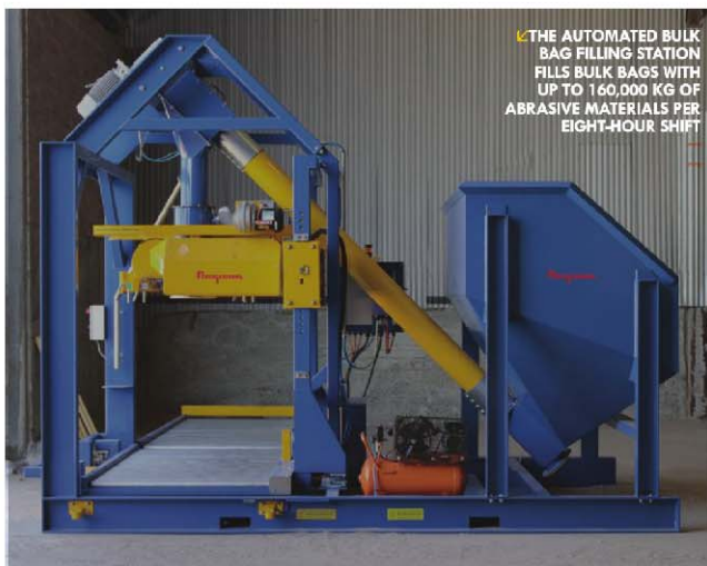
SKID-STEER LOADER DEPOSITS MINERAL SANDS INTO THE 2.5M 3 CAPACITY HOPPER WHILE THE SCREW CONVEYOR MOVES THE MATERIAL TO THE BULK BAG FILL HEAD.
