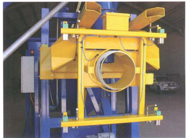
The Swing-Down fill head pivots to a vertical position, allowing the operator to safely and rapidly attach bag straps to filler latches while standing on the plant floor. Pushing one button inflates the material inlet against the bag spout, and initiates all automatic bag filling functions.
