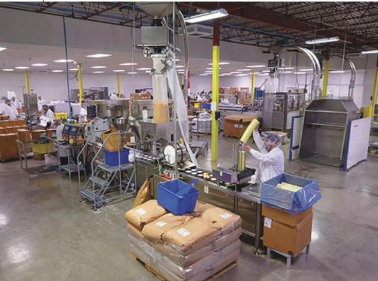
Because the tubular cable conveyors fully evacuate material, cleaning and product changeover can be accomplished in 15 to 20 minutes, says Kish. During changeovers, workers clean the TCC lines with antibacterial swabs and flexible sponges.
