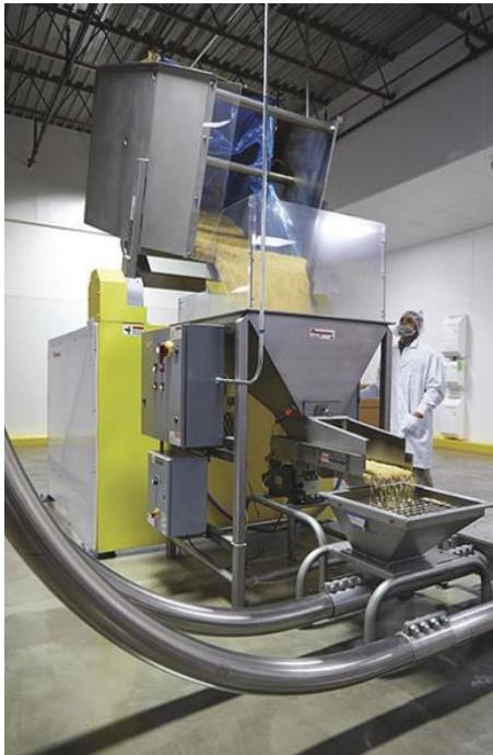
▶ **Open-box dumpers from Flexicon Corp. unload pasta from Gaylord containers. The pasta is then moved by tubular cable conveyors to minimize breakage and dust.** Source: Quality Pasta Company.
