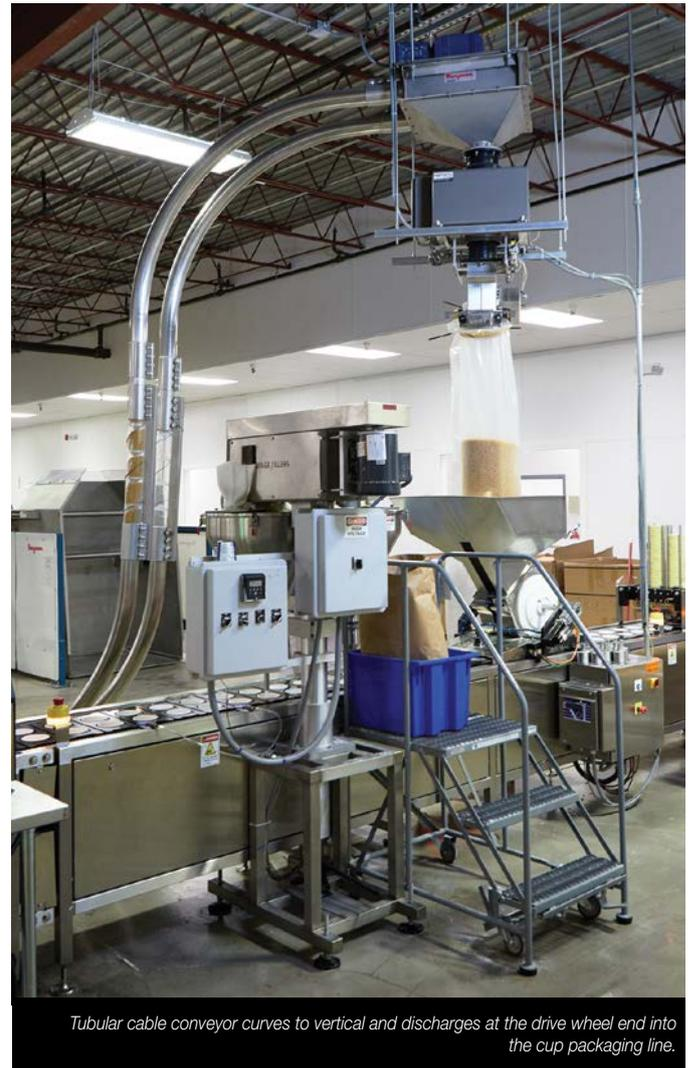
*Tubular cable conveyor curves to vertical and discharges at the drive wheel end into the cup packaging line.*
