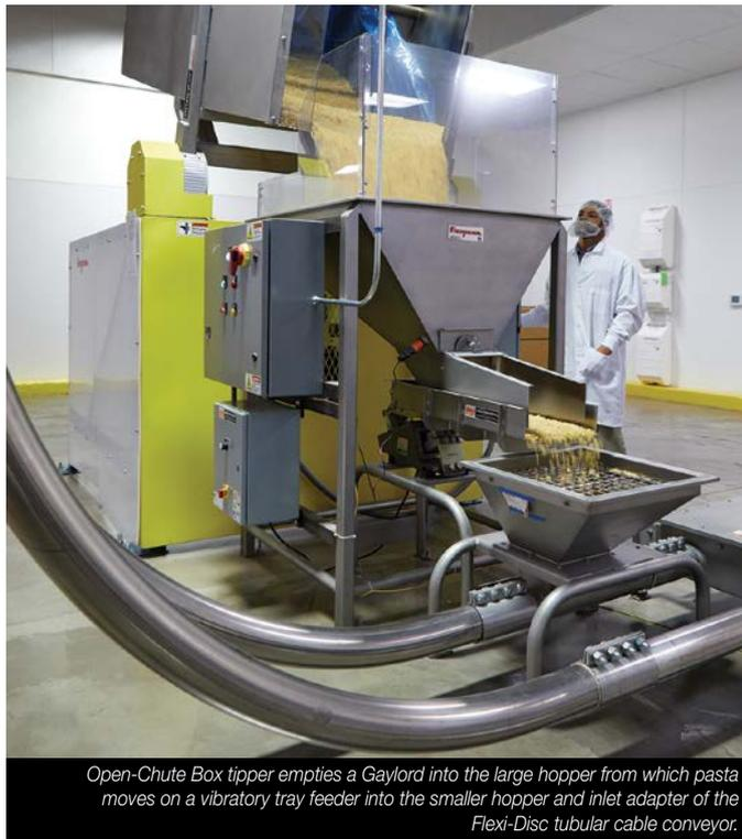
Open-Chute Box tipper empties a Gaylord into the large hopper from which pasta moves on a vibratory tray feeder into the smaller hopper and inlet adapter of the Flexi-Disc tubular cable conveyor.
