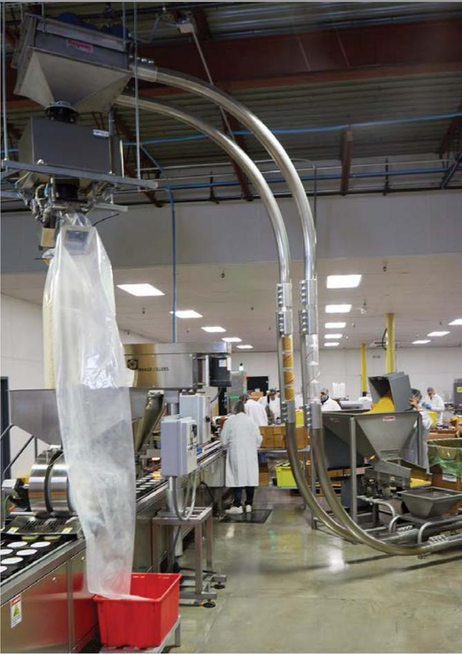
The two Open-Chute box tippers from Flexicon automatically raise and tilt the Gaylords, which discharge pasta into 227 litre hoppers. Pasta discharges from the hoppers onto vibratory tray feeders that control the rate at which material flows into the inlet adapter of each Flexi-Disc conveyor, also from Flexicon.
