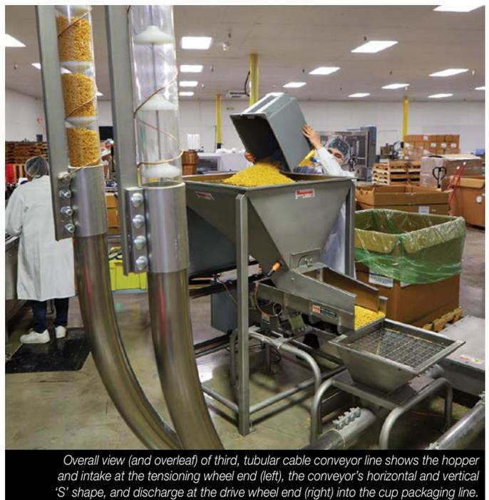
Overall view (and overleaf) of third, tubular cable conveyor line shows the hopper and intake at the tensioning wheel end (left), the conveyor's horizontal and vertical 'S' shape, and discharge at the drive wheel end (right) into the cup packaging line.
