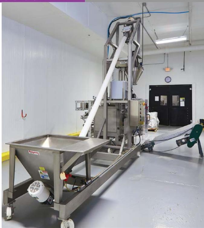
Portable "cheeser" line includes a 156 litre hopper and 4.6 m long Flexicon screw conveyor for packet packaging of cheese powder.
