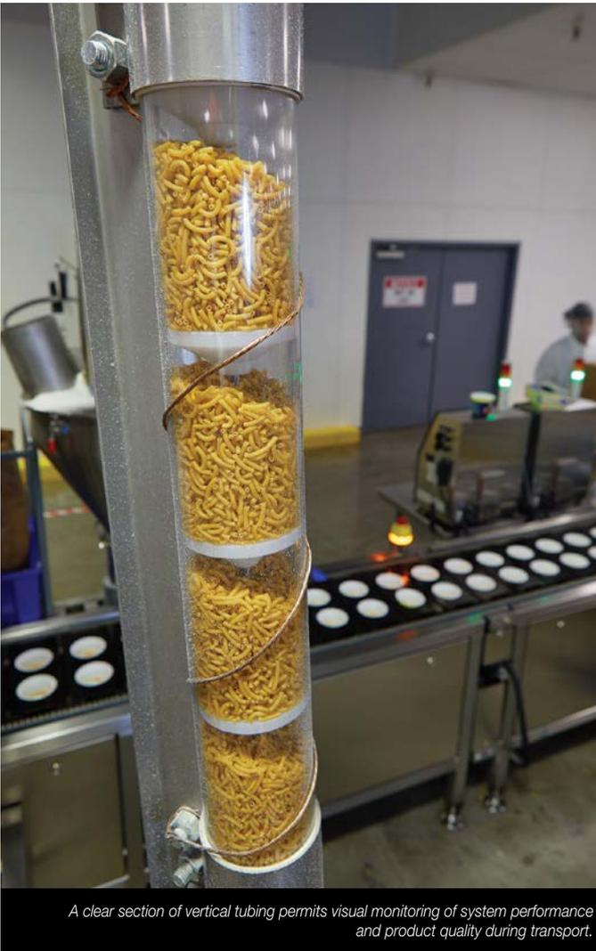
*A clear section of vertical tubing permits visual monitoring of system performance and product quality during transport.*
