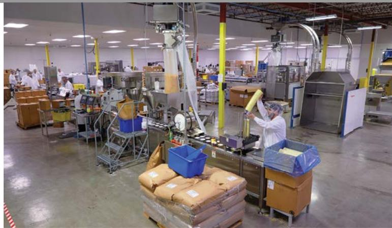
Three tubular cable conveyor circuits and two automated box tippers move brittle pasta to three sanitary packaging lines at high rates without product breakage or dust.
