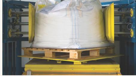
Hydraulic rams fitted with specially contoured end plates press opposite sides of the bag to loosen solidified powders. The turntable and bag rotate 90° to condition all sides, while the scissor lift allows conditioning at all heights.
