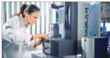
The Kinexus rheometer from Malvern Instruments - which offers extensive capabilities in advanced rheology and viscosity measurement - is currently playing an important role in research being undertaken by Germany's Clausthal University of Technology into the physical properties of drilling fluids (see p11).
