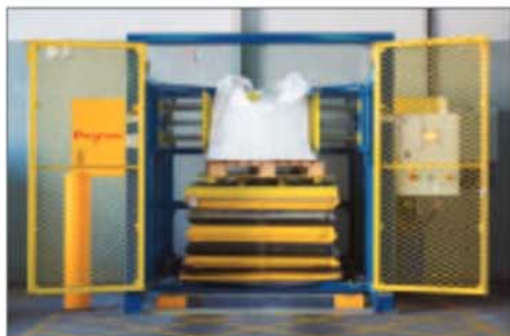
A scissor lift raises the bulk bag to a preselected height while hydraulic rams with contoured end plates press opposite sides of the bag to loosen solidified powders.
