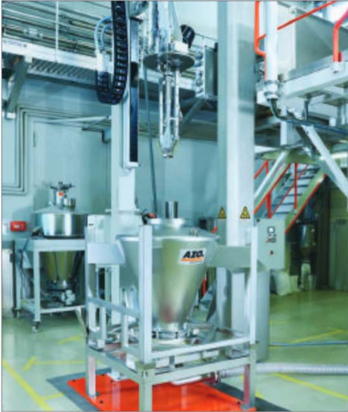
AZO can now offer a sophisticated system which is capable of dry cleaning the interiors of IBCs and similar transport/storage vessels; unlike with wet cleaning, problems and costs associated with disposal of contaminated or toxic wastewater are avoided, as described on p14.
