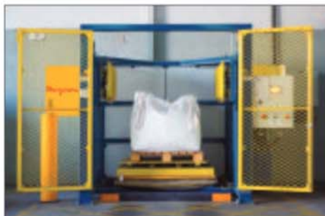
A scissor lift raises the bulk bag to a preselected height while hydraulic rams with contoured end plates press opposite sides of the bag to loosen solidified powders.
