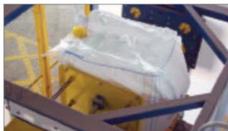
The turntable and bag rotate through 90 degrees to condition all sides, while the scissor lift allows conditioning at all heights; in addition to ensuring greater safety and enhanced quality of the raw materials, the Block-Buster has cut de-lumping time by 75%.
