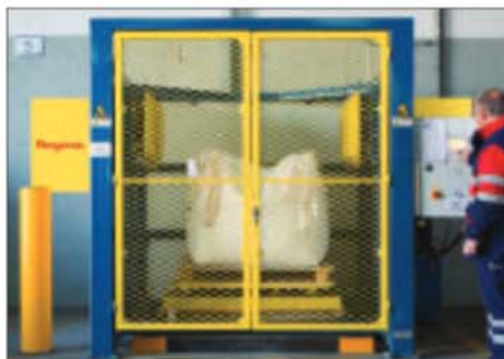
Once the safety doors are secured, the operator initiates the conditioning cycle.
