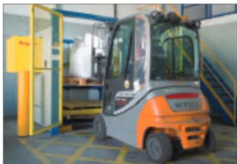
A bulk bag is loaded into the conditioner by forklift.
