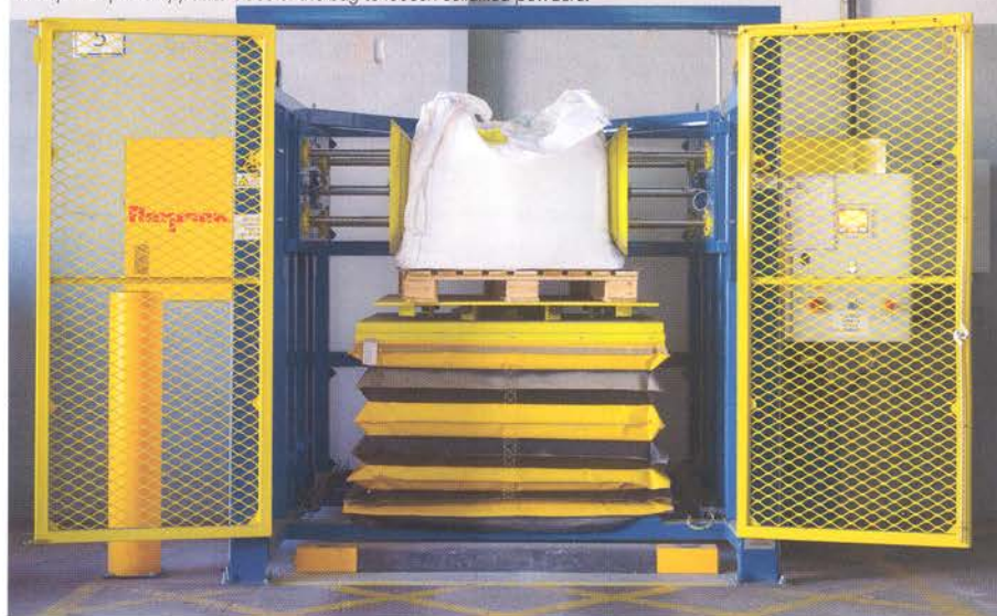
Scissor lift raises the bulk bag to a preselected height while hydraulic rams with contoured end plates press opposite sides of the bag to loosen solidified powders.
