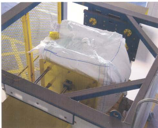
Hydraulic rams fitted with specially contoured end plates press opposite sides of the bag to loosen solidified powders. The turntable and bag rotate 90° to condition all sides, while the scissor lift allows conditioning at all heights.
