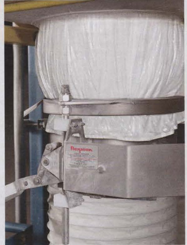
The operator opens the outer closure of the bag to access the bag spout which he connects to a dust-tight Spout-Lock clamp ring. Once the drawstring is released, material flows through the bag spout as a Tele-Tube telescoping tube maintains constant downward tension on the clamp ring, promoting complete discharge as the bag empties and elongates.
