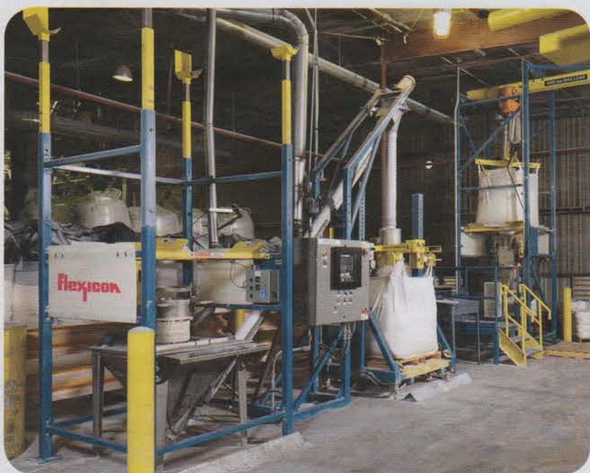
Two bulk bag dischargers, a flexible screw conveyor, a bulk bag filler and programmable controls allow re-bagging of PVC modifiers into bulk bags of three sizes and 50-lb sacks, efficiently and dust-free.
