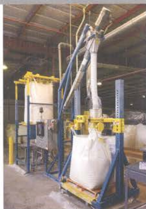
The flexible screw conveyor transfers material from the bulk bag discharger (rear) to the bulk bag filler (foreground). A height-adjustable fill head accommodates bulk bags in any of three sizes used by the company.
