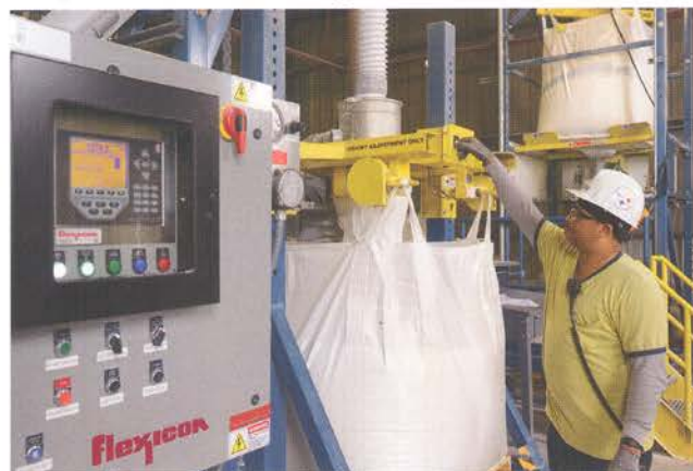
The flexible screw conveyor transfers material from the bulk bag discharger (rear) to the bulk bag filler (foreground). A height-adjustable fill head accommodates bulk bags in any of three sizes used by the company.
