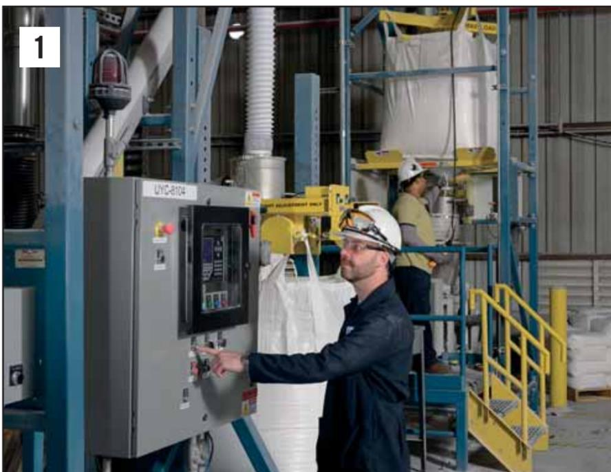
1) Operator in foreground initiates a bulk bag filling cycle while operator in background loads a bulk bag into the discharger frame using its electric hoist and trolley
