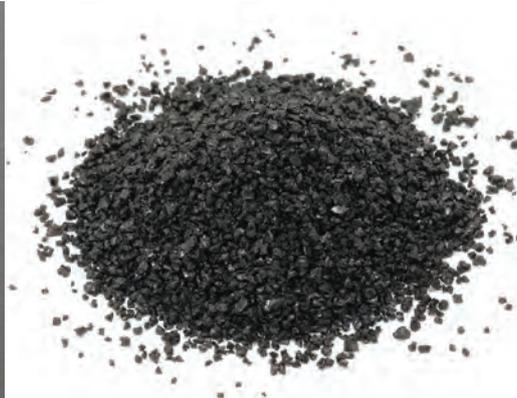
**Silicon powder is the main ingredient in Nexeon's manufacture of silicon anodes.**
