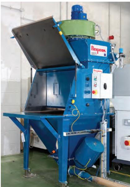
Silicon powder and additives are manually emptied into the bag dump station and floor hopper. The station includes a bag tray support and dust collection through two cartridge filters. Powders flow from the hopper outlet through a pickup adapter into the pneumatic conveying line.
