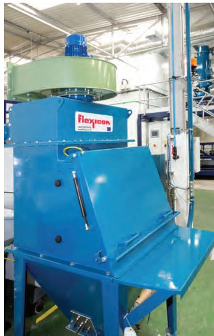
Powders move from the bag dump station through the pneumatic conveying line to the filter receiver (rear) in the main processing area. Fully enclosed system prevents the escape of dust.
