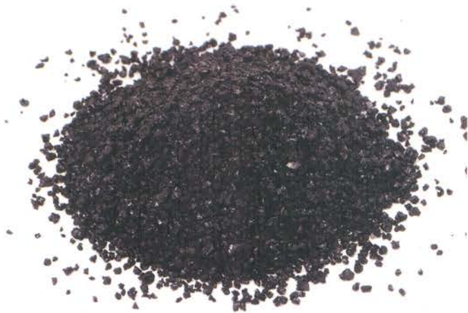
Silicon powder is the main ingredient in Nexeon's manufacture of silicon anodes.
