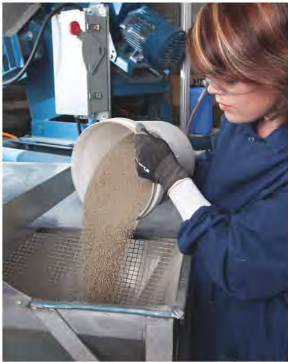
The flexible screw conveyor moves the pellets at a 45 degree incline to the fluid bed dryer.
