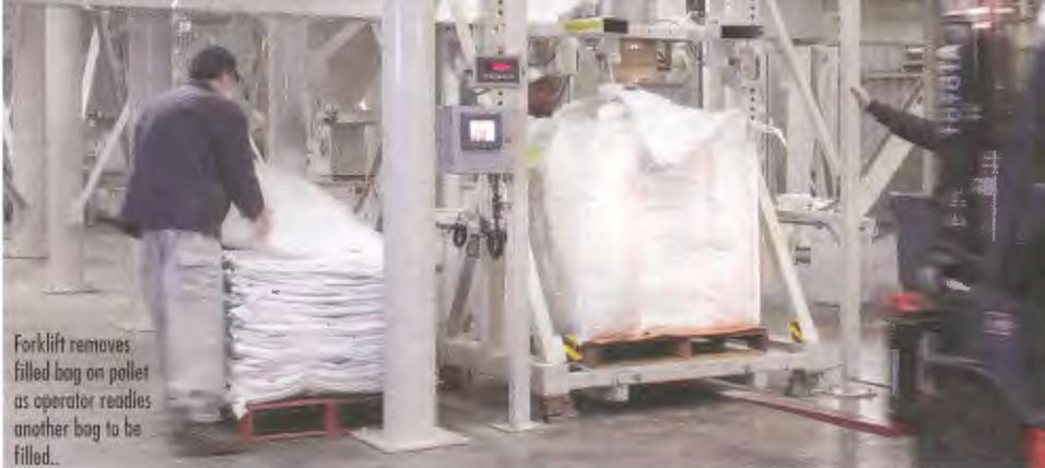
Forklift removes filled bag on pallet as operator readies another bag to be filled.
