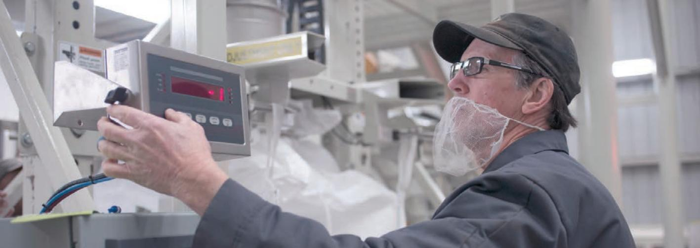
Once the operator connects the bag and pushes “start,” a PLC automates the filling process, closing the dome valve when the bag reaches its target weight.
