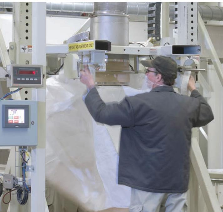
Operator attaches bag loops to retractable bag hooks that suspend the bag during filling.
