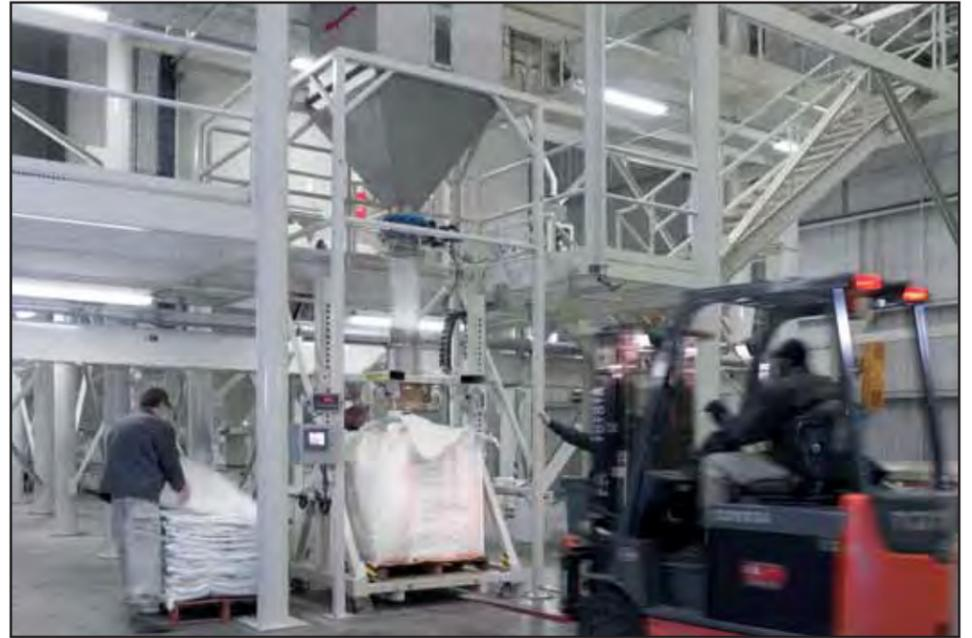
Forklift removes filled bag on pallet as operator readies another bag to be filled
