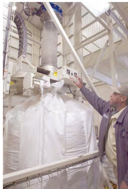
Operator inflates the bag, removing creases prior to filling
