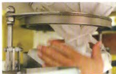
Once a bag is hoisted into position, an operator pulls the bag spout over a Spout-Lock clamp ring, which creates a secure, dust-tight connection between the clean side of the bag spout and the clean side of a Tele-Tube telescoping tube, which maintains constant downward tension to promote complete discharge.
