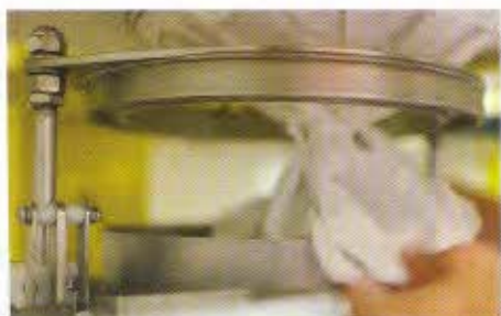
Once a bag is hoisted into position, an operator pulls the bag spout over a Spout-Lock clamp ring, which creates a secure, dust-tight connection between the clean side of the bag spout and the clean side of a Tele-Tube telescoping tube, which maintains constant downward tension to promote complete discharge.
