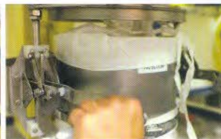
Once a bag is hoisted into position, an operator pulls the bag spout over a Spout-Lock clamp ring, which creates a secure, dust-tight connection between the clean side of the bag spout and the clean side of a Tele-Tube telescoping tube, which maintains constant downward tension to promote complete discharge.
