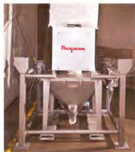
▲ Limited headroom requires a forklift to suspend bulk bags above the lower half of this split-frame Bulk-Out® bulk bag discharger. Once the room is enlarged with a higher ceiling, bulk bags will be loaded at floor level into the top half of the split-frame, which will then be forklifted with bag intact, onto the lower half of the frame, within centimetres of the ceiling.
