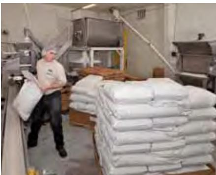
opening is drawn into the dust collector and deposited on the outer surfaces of two cartridge filters. Periodic blasts of compressed plant air blown onto the filters dislodge the dust particles, which fall into the hopper. The process is continuous with compressed air blasts alternating between the two filters.
