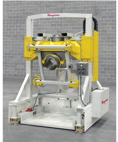
*Flexicon's TWIN-CENTERPOST™ Bulk Bag Filler with SWING-DOWN® fill head and low profile deck allows safe, rapid spout connections and removal of filled bags using a pallet jack.*
